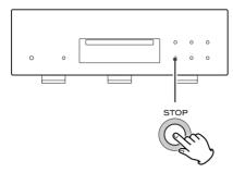
When playback is stopped, hold down the STOP button for more than 2 seconds and release it when "i.60958", "i.PCM" or "i.OFF" appears on the display.
